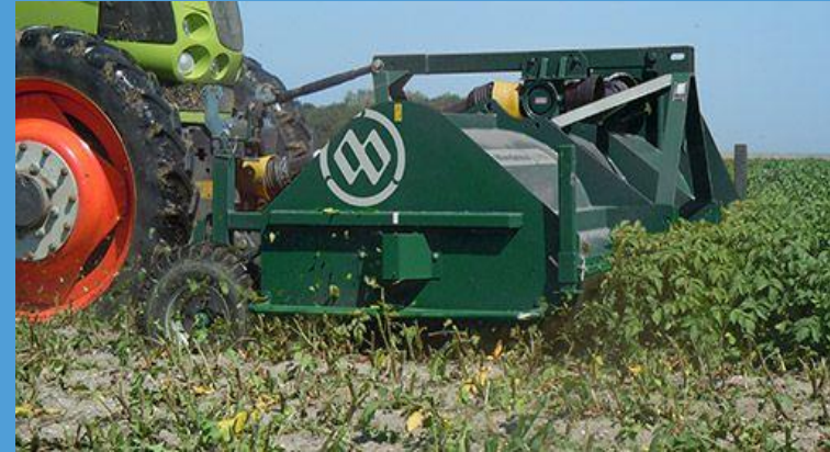
Flailing (haulm topper): Infections of haulms (via flails), roots and tubers (via tyres or indirectly via infected haulms)
