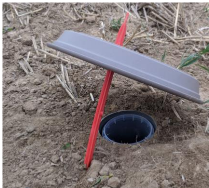
A Barber ground trap to catch arthropods crawling on the soil surface.
